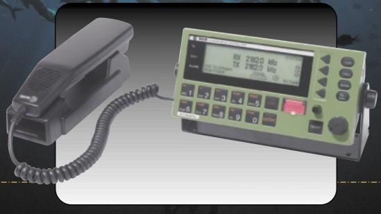
SAILOR System 4000 150W MF/HF is part of SAILOR's compact System 4000 solutions. It is an integrated MF/HF radio with voice and DSC built into one unit, from one of the leading and most experienced manufacturers of maritime communications equipment in the world.
