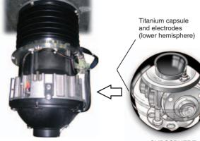
Anti-vibration mechanism (top) and Container (bottom)
