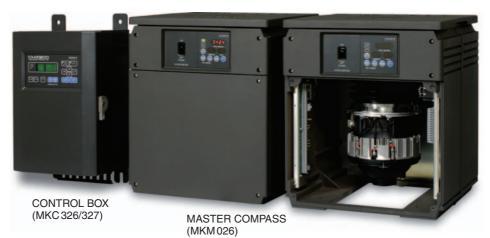
A gyrocompass detects the true north by means of a fast-spinning rotor, which is suspended with no friction and is influenced by gravity and rotation of the Earth. A gyrocompass consequently indicates a ship's heading.
